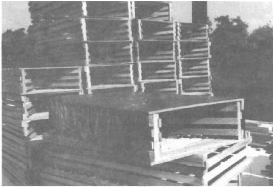
FIGURE 15 - Second generation 24" x 48" x 8" den-trap covered with black sheeting on all but the entrance end(s).
