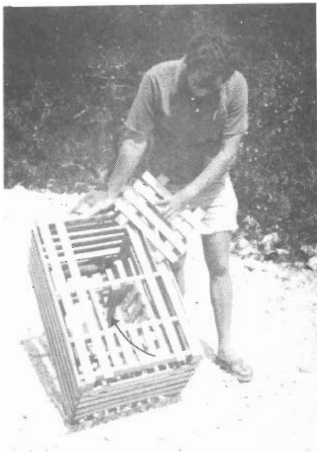
FIGURE 7 - A conventional spiny lobster trap with the addition of a 1\frac{1}{4} ' x \frac{3}{8} " climbing slat extending down to the bottom of the trap along the side of the throat. The person in the photograph is holding the access panel in his left hand.
