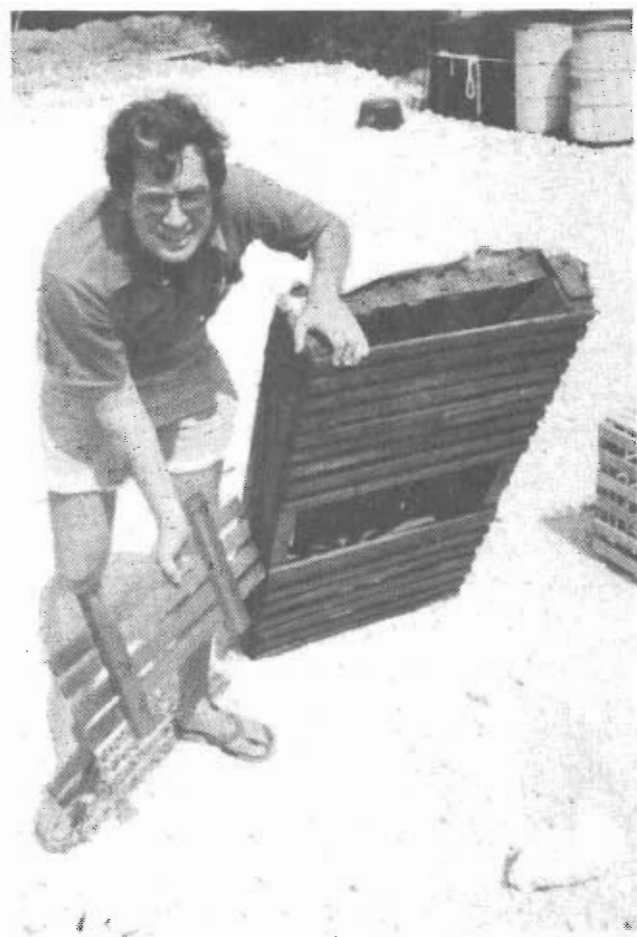
FIGURE 13 - Highly modified habitat-trap designed to reduce the need for climbing and to provide dark shelter. The dimensions for this first generation trap are 24" x 48" x 6" with a single access funnel. The habitat-trap is completely covered with black sheeting. The person in the photograph is holding the access panel in his right hand.
